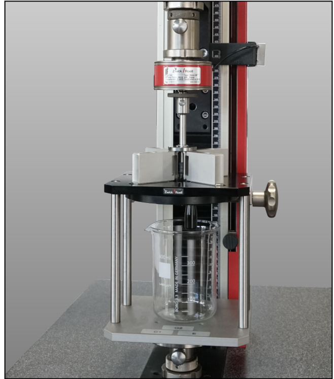
Test fixture for determining breakaway force and glide force, with carpule mounting
